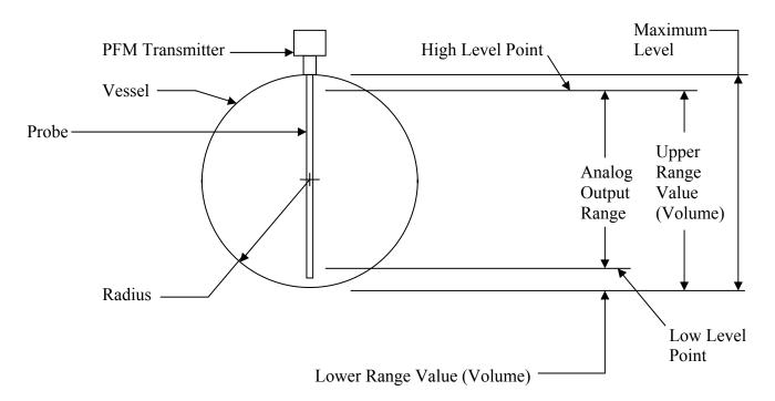
Determine the Maximum Level. This is the highest point that can possibly be measured. This is usually, but not always, the same as the tank height. Fill in the value below.
